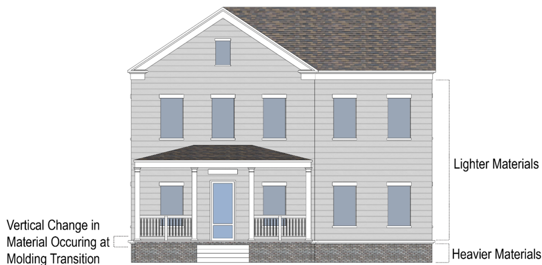
Figure 27-243-1: Residential building material and details
