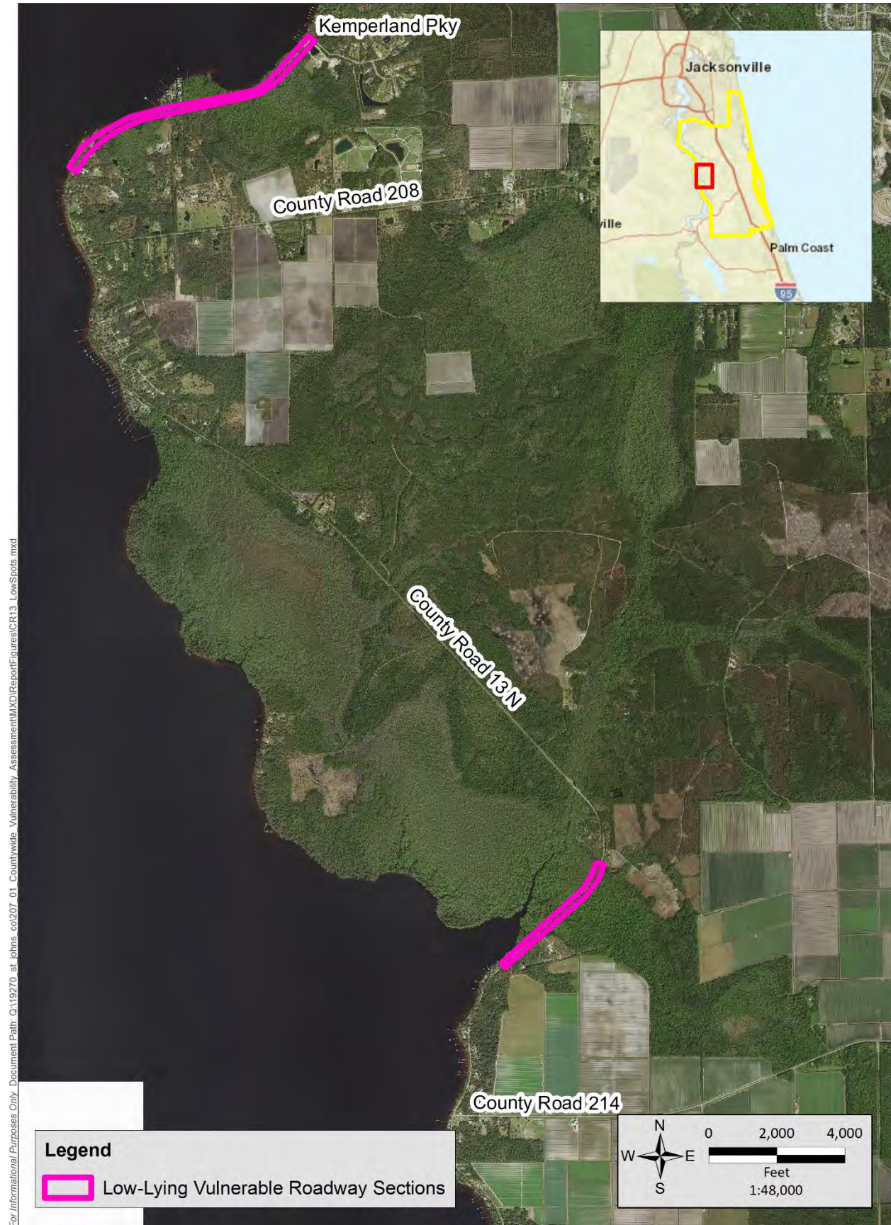
Figure 8 Low-Lying Vulnerable Sections of CR13N
